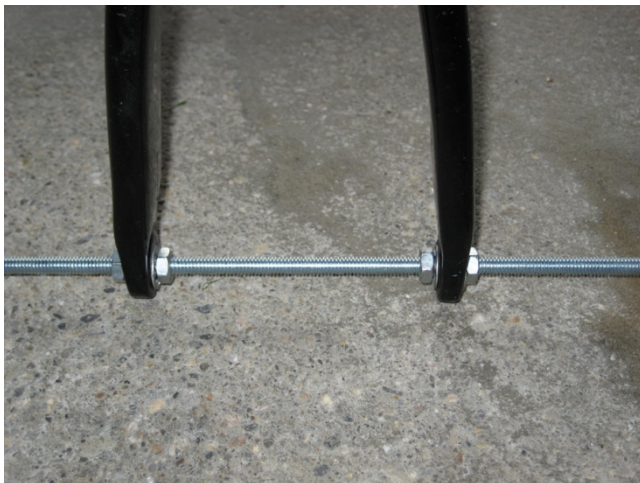
Figure 1: Fork Mounted to 6' Rod, Secured with Washers and Nuts
