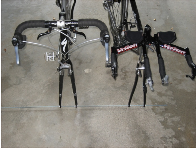
Figure 2: Bikes Mounted on 6' Rod, Forming a Stable Platform
